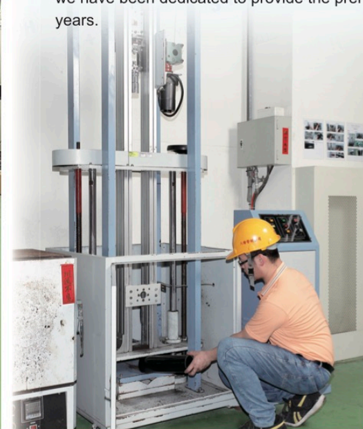
耐落錘測試實驗裝置 Falling hammer resistance device
