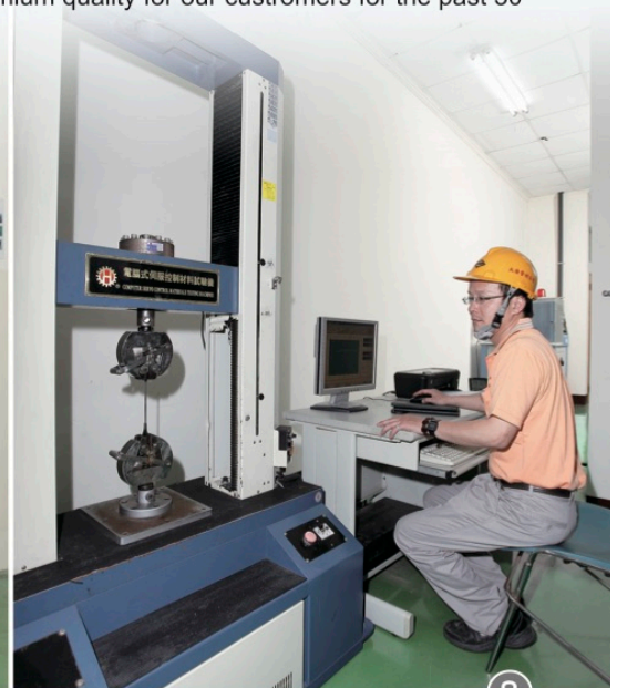
拉力材料試驗機設備 Tension strength testing equipment
