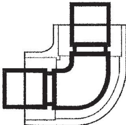
DC 90° Ells are made from standard pressure fittings by DFP in designated material and schedule selected. Included are separate internal carrier and external containment fittings of the same configuration.
